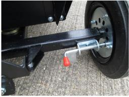
5.2.3 Place pin through turnbuckle and tighten
